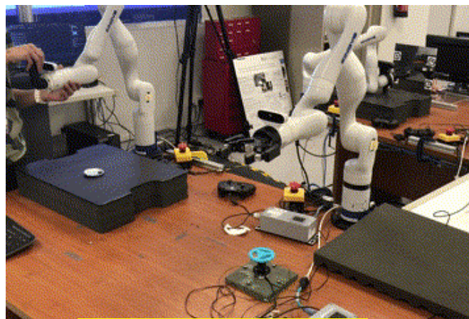
Valve turning with axial misalignment
